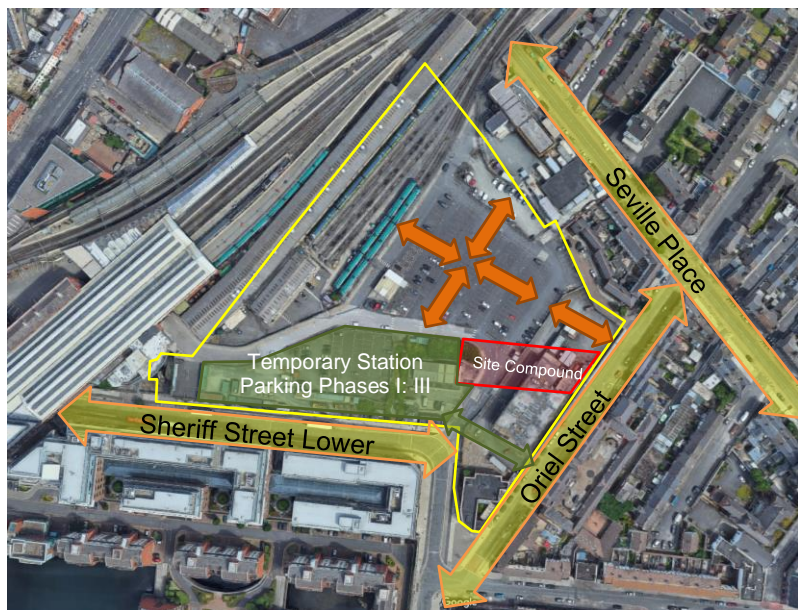
Figure 6: Site Set Up Phase I, II & III
