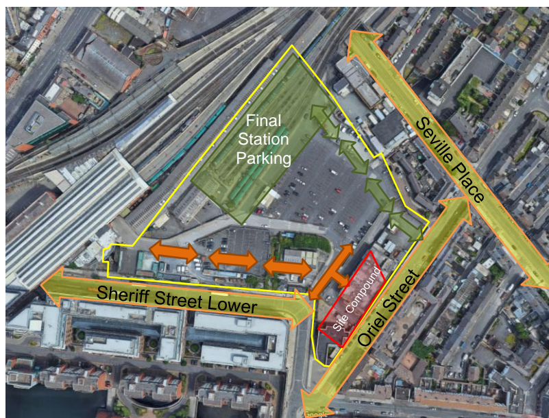
Figure 7: Site Set Up Phase IV, V & VI
